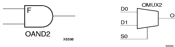
Figure 21: AND & MUX Symbols in XC4000X IOB
